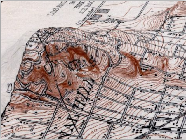
Figure 0-3. Historical topographic map draped over topography extracted from it onto a digital elevation model.
